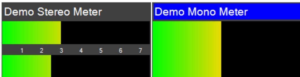
**Label Above Meter with dbFS** is as above but will show a dbFS scale on the stereo meter (not on the Mono meter).
