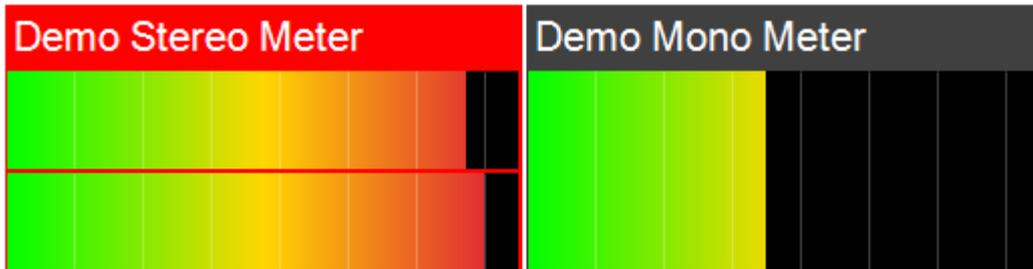
The **Border Style** menu selects between all of the different designs of the meters. Default is "3D". Not relevant to PPM Meters.
