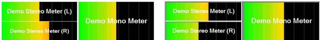
**PPM Scale Top / dbFS Scale Top** will show a scale on a grey background above the meter. "Top" changes to "left" when the meters are Vertical Bars.
