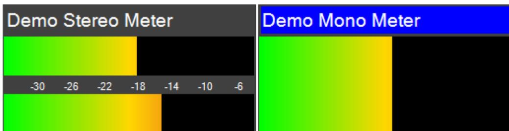
**Display Meter Scale Lines** lets you choose between PPM markings every 4db, block markings every db, or no markings. This can be used with or without actual number scales being displayed with some of the Border Styles. PPM markings is the default. Not relevant to PPM Meters.
