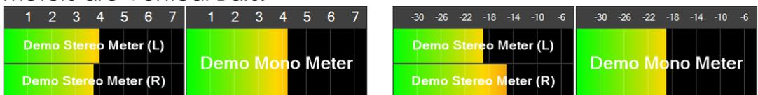
**PPM Scale Middle / dbFS Scale Middle** will show the scales in between the left and right meters. Note that with a mono meter no scale will be shown.
